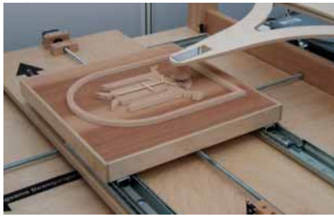
Das Modell eines Rasterkraftmikroskops (AFM) tastet das Münchner Stadtwappen ab. | The model of an atomic force microscope (AFM) scanning Munich's coat of arms.
