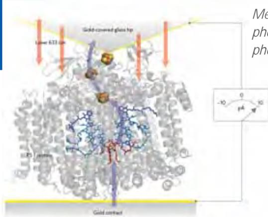
Measurement of the photoelectricity of the photosystem I - proteins
