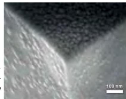
Picture of scanning electron microscopy of the glass tip after coating it with about 20 nm of gold
