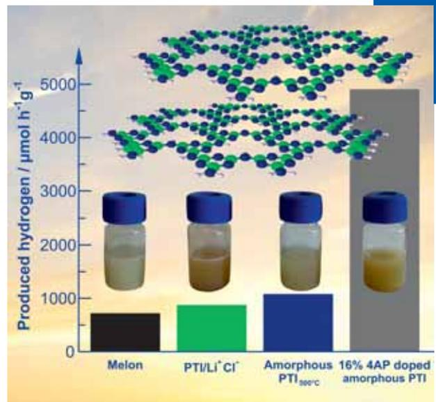
Light-induced hydrogen evolution by different carbon nitride photocatalysts
